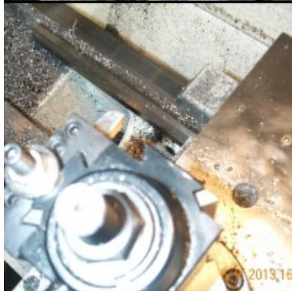
Before relief was ground (in the last image you can see the form of the cutter in the shadow it casts just to the right of the blank)
