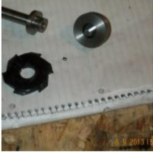
Wanted to make a [Delrin 120 tooth idler gear for my PM14x40 lathe](#). A few years back i made a small 24 tooth spur gear for a 3-1 multi-machine (Mill/Drill/Lathe) so i could add a thread dial, that gear was made by a single point cutter ground to the correct angle and looked kind of like a fly cutter... For this 120 tooth project i wanted to make a multi-edge cutter that would create an Involute Gear. Did alittle research found the radius which i needed and did the following:
