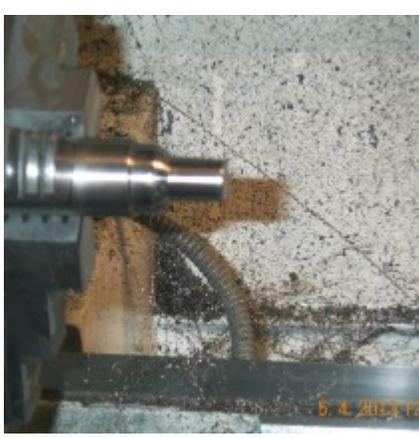
Heres the rod with the Delrin guide. Turned the guide OD over size, drilled and then taped it 3/8-16 and cut it off, then screwed it to the end of the 1/2 rod and over tightened it over the shoulder alittle, then turned the OD to size, faced & back faced it square.
