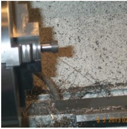
During a test assembly i found that there was "suction" (back presser ???) while sliding the sleeve up and down the rod so i drilled two "air holes", one right in the end of the M16 taper and the second through the side of the sleeve towards the back near the cap. The two air holes made a big difference, the "plunger" now slid nice and smooth.
