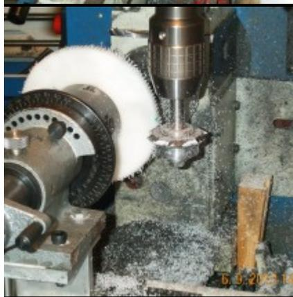
Gear done. The thin washer goes on the machine first, the bore is a tight fit to the "bolt" which the gear slide over (the bolt seam to be under size, 10MM on the low and the old gear and current bearings are sloppy) and the end which the gear will be seating on has a taper to it so it "centers" the bearing, i did the same to the knurled nut and it seamed to work out pretty good.
